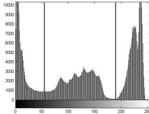
**Fig. 4:** A histogram of the blue channel with local minima (level 54 and 197)
