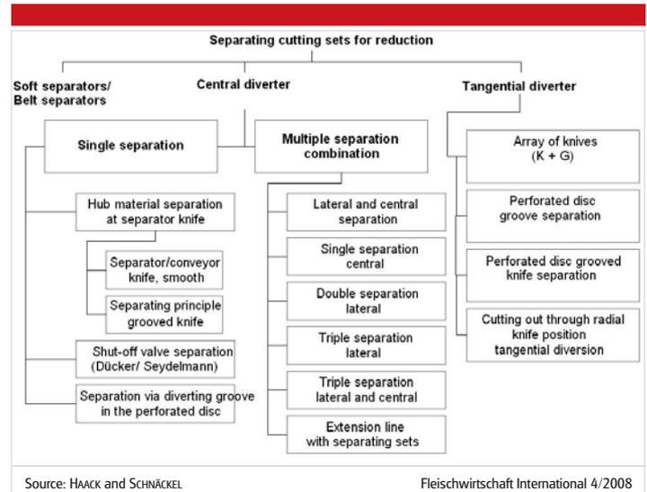
Fig. 4: Classification of the reduction separator sets on the basis of their operating principles
