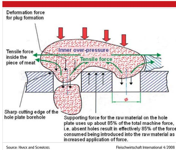
Fig. 3: Schematic representation of the meat behaviour at the perforated disc as the basis for outflow operations
