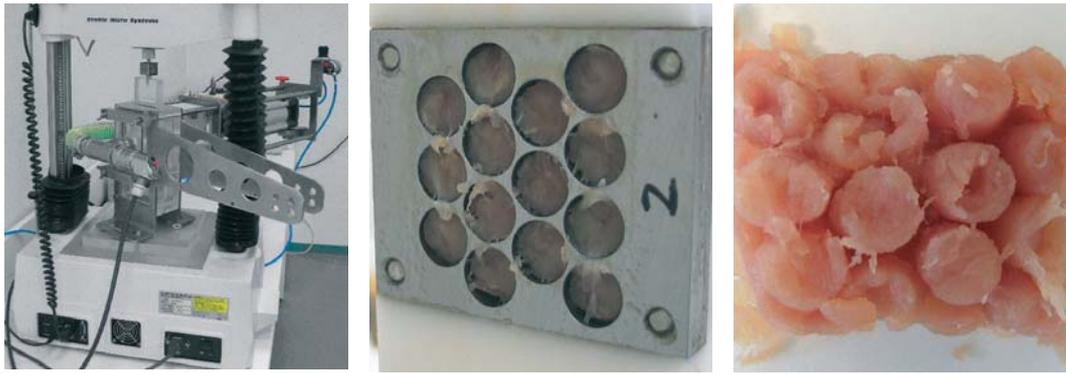
Fig. 1: Texture analyser TA HDplus with cutting system (left), cutting punch with perforation and plug formation
