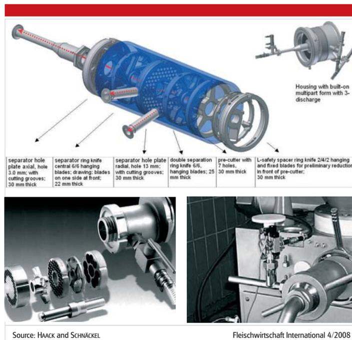
Fig. 5: Representation of different kinds of separator set devices
