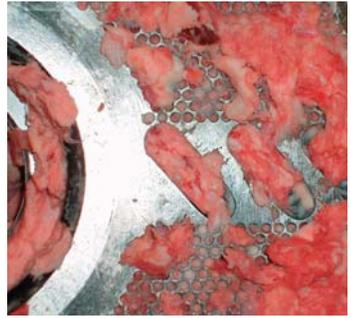
Fig. 3: Perforated disc W300 – hole diameter 2.4 mm with cutting grooves (left) and in operation (right) (Power Tools, Germany)
