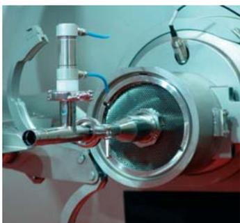
**Fig. 2:** Cutting set with central discharge with pneumatically controlled cutting setting without support cross (Power Tools, Germany)
