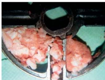
Fig. 4: Grading knife with side discharge above the knife ring
