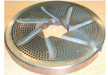
**Fig. 1:** Perforated disc with discharge channels (Seydelmann, Germany)
